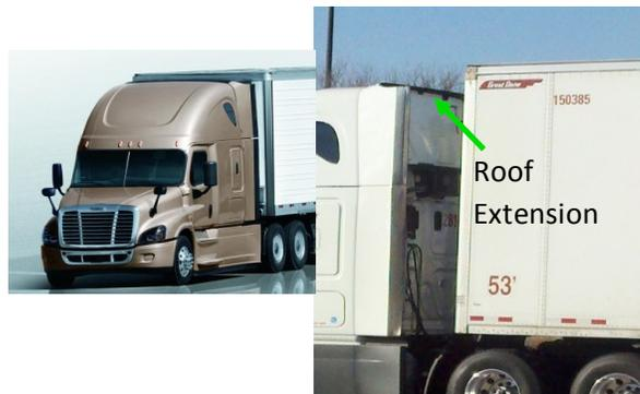
Figure 25 Freightliner Cascadia Roof Extension (Freightliner)
