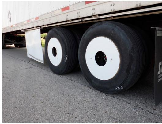
*Figure 45 Solus Wheel Cavity Cover*
