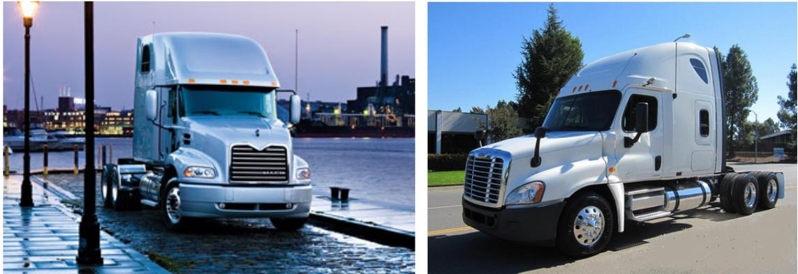
Figure 34 Examples of Otherwise Aerodynamic Tractors but w/o Chassis Fairings
