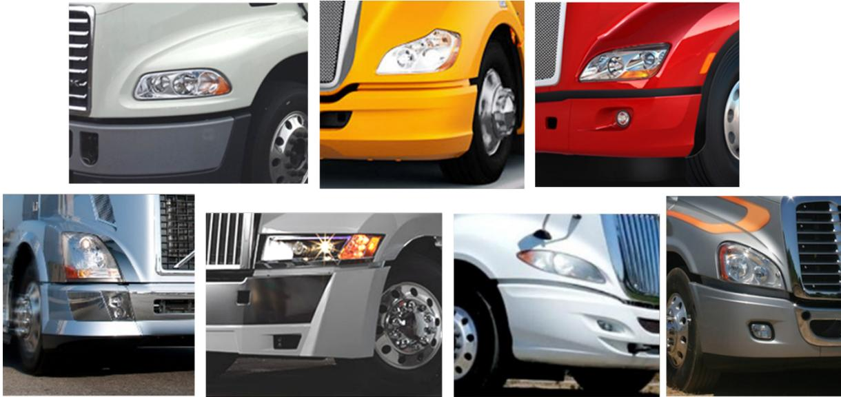
Figure 43 Aerodynamic Headlamps and Bumpers Conform to Hood Shape – Volvo VNL780, Western Star 5700, Navistar ProStar, Freightliner Cascadia, Peterbilt 579, Kenworth T680, Mack Pinnacle
