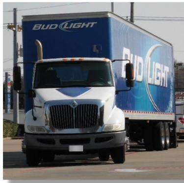
Figure 14 Example No-Aero Device Day Cab
