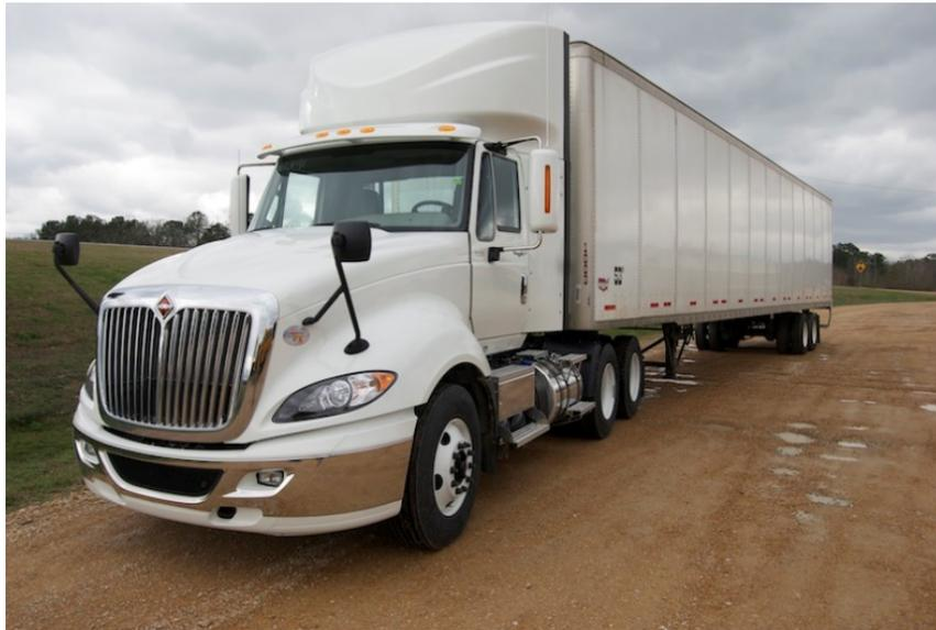
*Figure 38: Similar Tractor with Cab Extenders and Roof Fairing*
