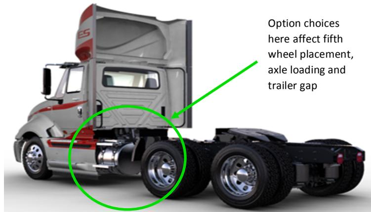
Figure 20 Chassis Option Choices May Affect Optimum Aerodynamics (Navistar)
