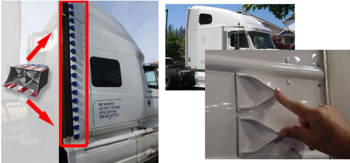
Figure 57 VorBlade and Air Tab Aftermarket Aero Devices
