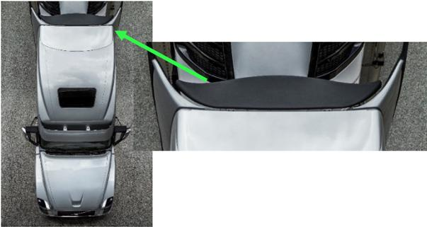
Figure 28 Volvo VNL680 Roof Extension (Volvo)
