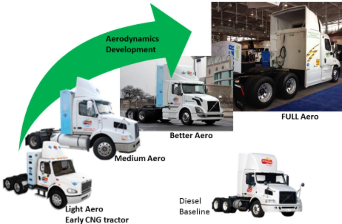
FIGURE 60: CNG Tractor Aero Evolution
