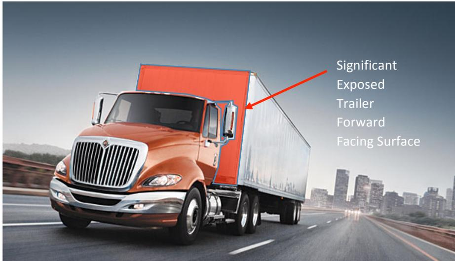
*Figure 37: Unfaired Day Cab Exposes Blunt Trailer Top Front and Sides to Airflow*
