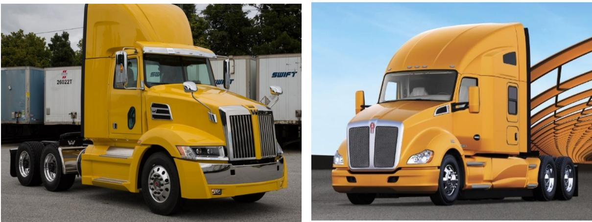
Figure 6 Day Cabs (left) and High Roof Sleepers (right) (Western Star & Kenworth)
